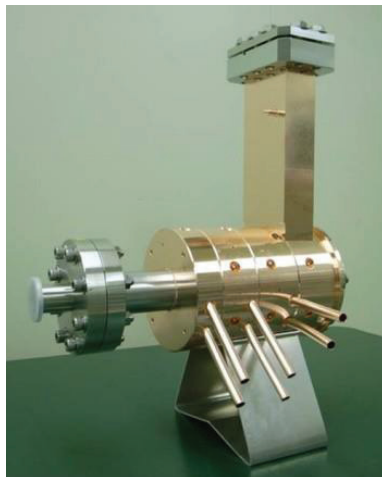
Room Temperature cavity for FEL
