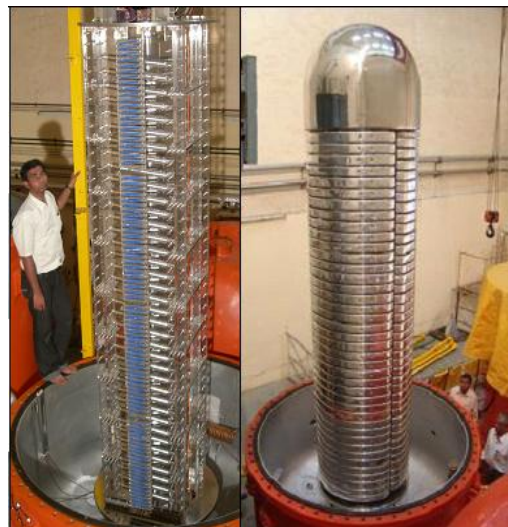
Fig. 3: Components of 3 MeV DC Accelerator
