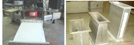
Figure4: Left 352.2 MHz circulator under tests. Right WR 2300 waveguide transitions and sections.
