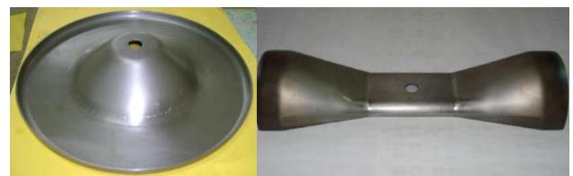
Figure 5: (a) Left – End Wall formed in niobium. (b) Right – Half Spoke formed in niobium and after machining the edges and ends.
