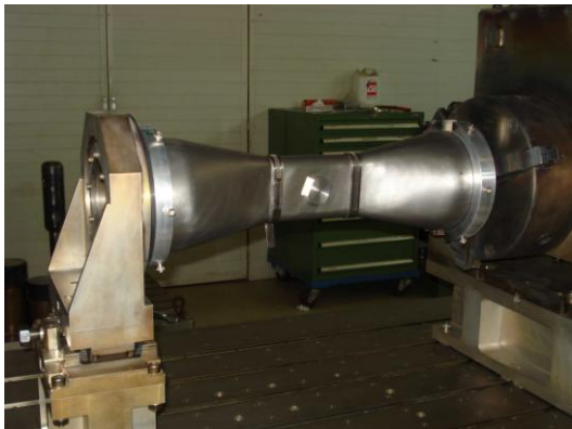
Figure 6: Electron beam welding setups showing, (a) above – outer shell, (b) below – spoke halves.
