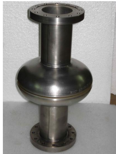
Figure 7: 1.3 GHz Tesla-type niobium single cell cavity.
