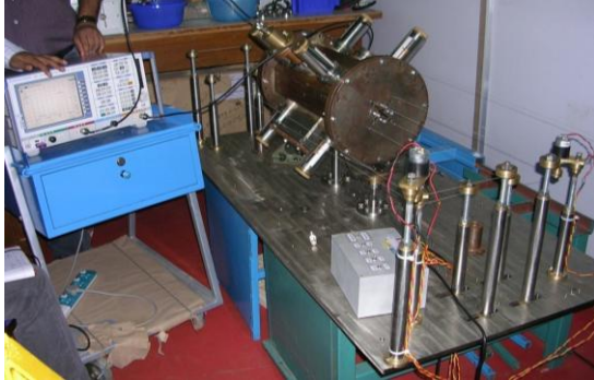
Fig. 5. Bead pull measurement setup.
