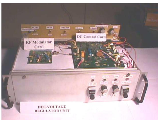
Fig.9. Dee Voltage Regulator Unit
