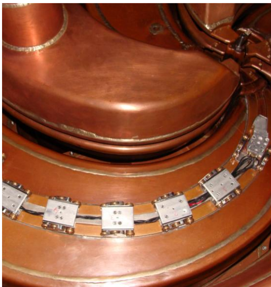
Fig. 6. The train like movement of the main probe on the hill section which measures current versus radius. The picture also shows the dees and the centre region at top right corner
