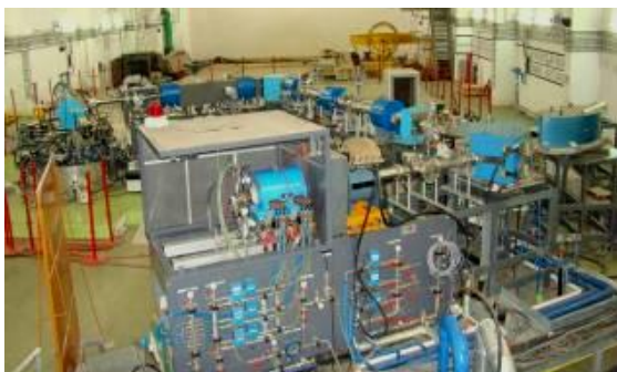
Fig. 4 Installed ECR Ion Source and Injection Line
