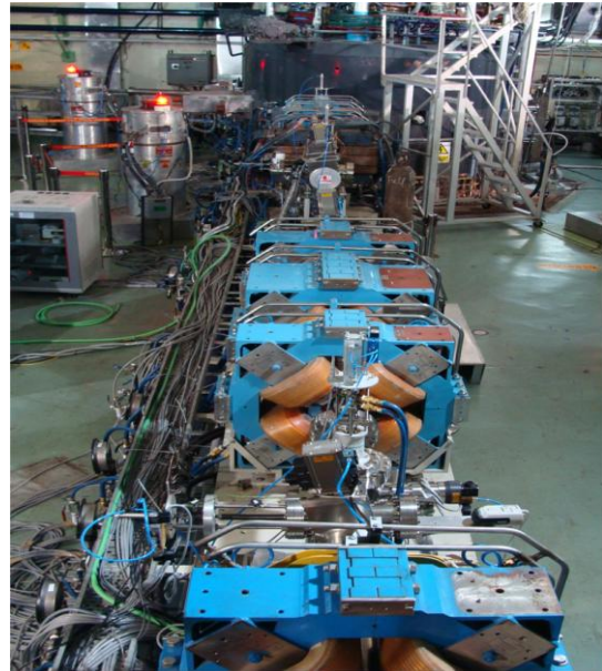
Figure 7. The external beam line leading to experimental station #1 in cave I
