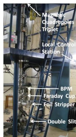
Figure 1: The new foil stripper near the object point of the 1.8m radius analyzing magnet of the 15 UD Pelletron.
