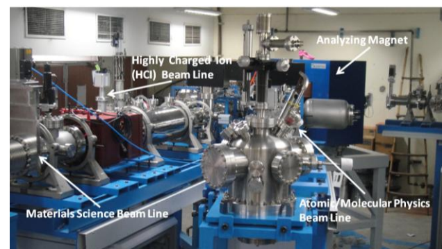
Figure 3: The new low energy ion beam facility (LEIBF) having ECRIS on a 400kV platform and three beam lines.
