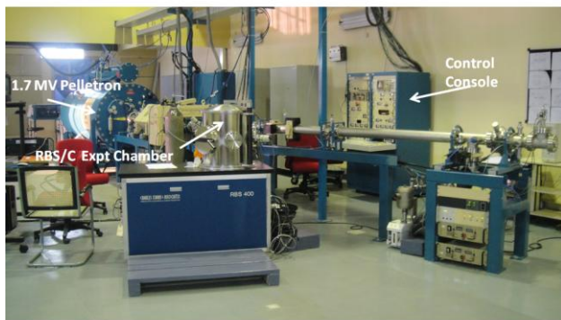
Figure 2. The 1.7 MV of Pelletron with Rutherford back scattering (RBS) and channelling facilities.
