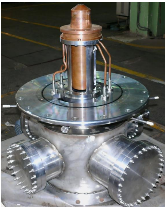
Fig. 4. Assembly of ECR proton source
