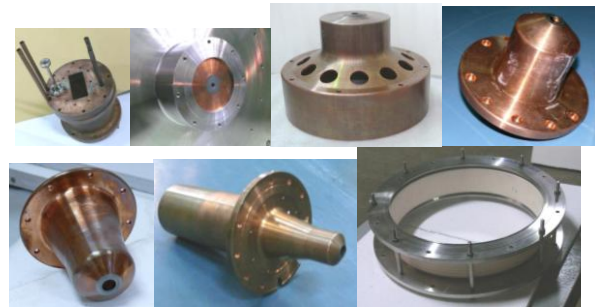
Fig. 2. Extractor electrodes and plasma chamber
