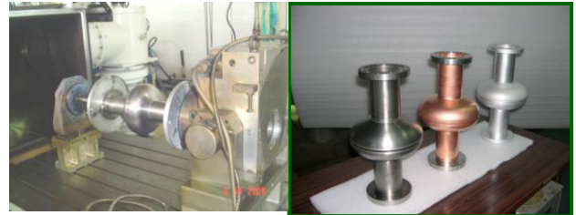
Figure 1(a): Final equator welding setting at IUAC, EBW facility. Figure 1(b): prototype single cell cavities in (r to l) Al, Cu & Nb.
