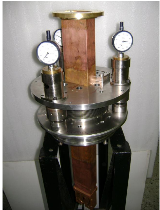
Figure 3: Mock-up assembly of RF Input unit on support
