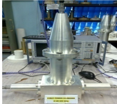
Figure 1: 2- Way RF power Combiner at 352MHz
