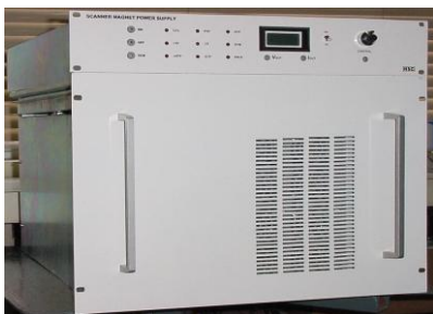
Figure 1: Photograph of scanning magnet power supply
