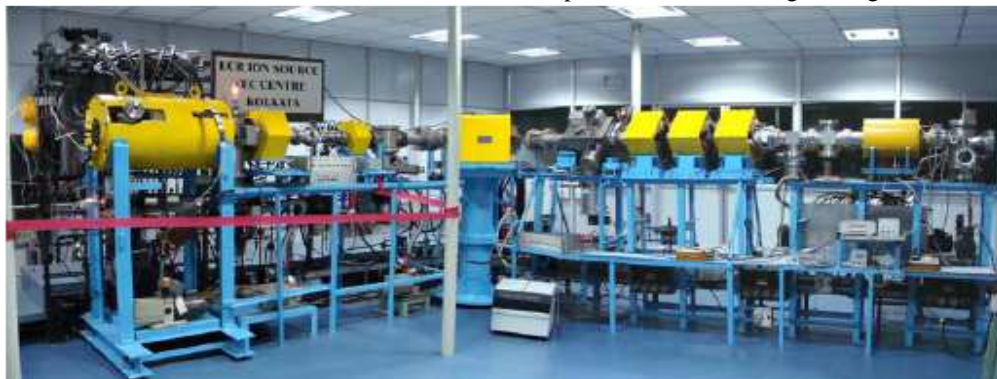
Figure 1: Layout of ECR-based Low Energy ion Beam Facility
