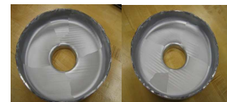
Figure 3 (b): Niobium large grain half cells.
