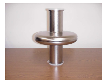
Figure 3(a): Fine grain single cell Niobium Cavity.
