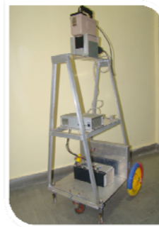
Fig. 1. The mobile robot with a gamma and neutron survey meter mounted on it.
