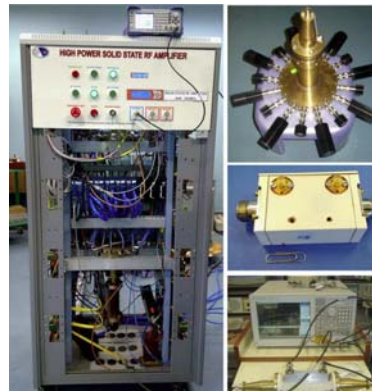
Figure 2: 4-kW amplifier at 352 MHz showing amplifier, power combiner and directional couplers.
