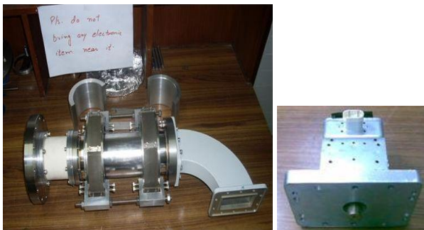
Figure-4: (Left) Plasma chamber with permanent magnets coupled to the extraction flange and waveguide; (Right) View of magnetron used for powering the ion source
