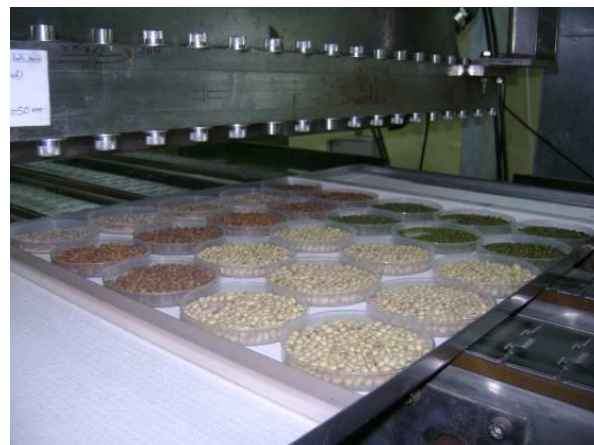
Figure 2: Tray with seeds on the conveyor belt.
