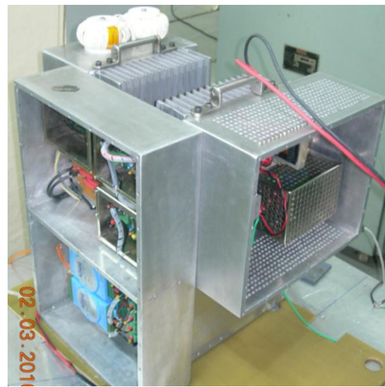
Figure 3: Photograph of Gun Power Supplies with Electromagnetic Shielding.
