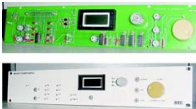
Fig. 5. Local Control Panel for Magnet Power Supply
