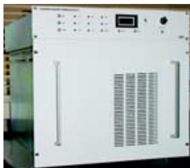
Fig. 2. High Current Scanner Magnet Power Supply
