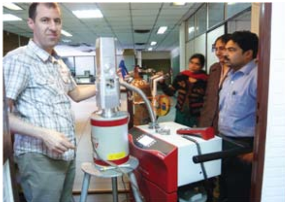
Fig. 10a: A Clover detector being repaired
