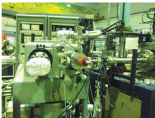
Fig. 31. Spectrometer coupled with the beam line.
