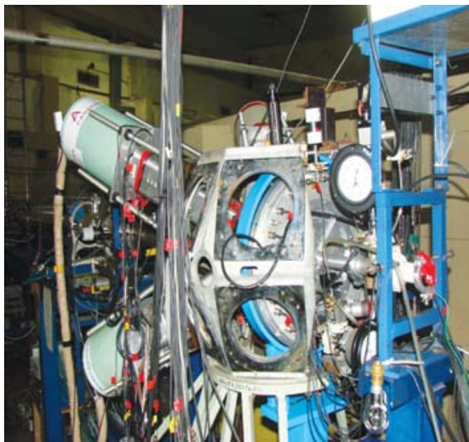
Fig. 11. A large area PPAC with four Clover detectors mounted on GDA structure.
