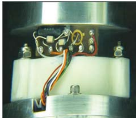
Fig. 10b: A FET replaced in a HPGe detector.
