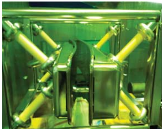
Fig. 15 The electrodes of ED (HYRA) set up in a clean room
