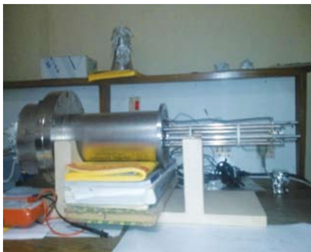
Fig. 8. Plunger device for INGA, reassembled with new DC micro-motors.
