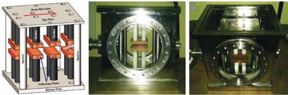
Figure 2.1.13: The mechanical assembly of TWC, (a) Inner Assembly, (b) side view, (c) Top View
