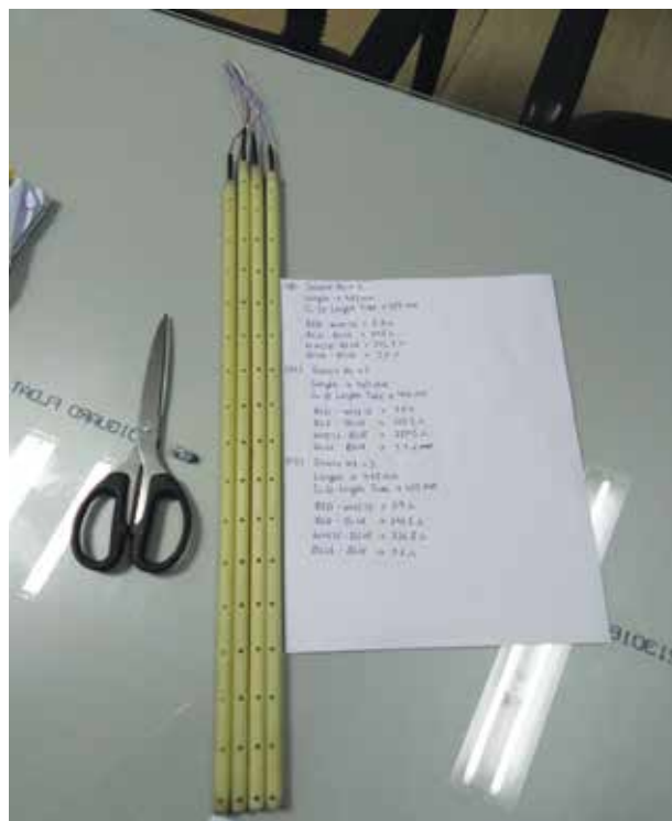
Fig. 3.1.9: A few of the LHe level sensors made at IUAC, some of which have replaced the existing AMI level sensors which were damaged during handling.
