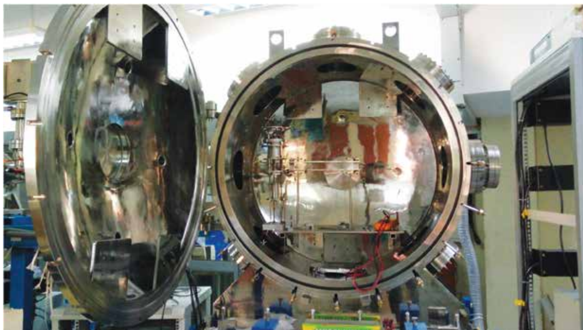
Figure 1.3.6: Time of flight spectrometer installed in the new chamber
