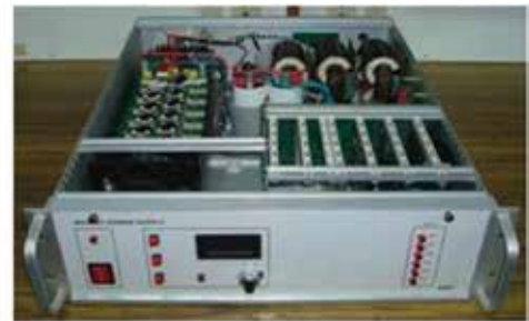
Photograph of the \pm 10 A bipolar LCPS
