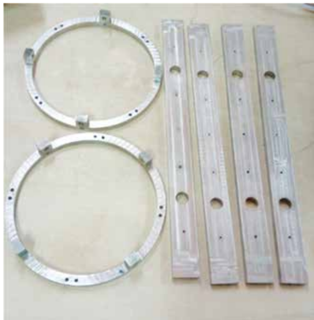
Figure 1.3.5: The fabricated inner parts of an Electrostatic Steerer.
