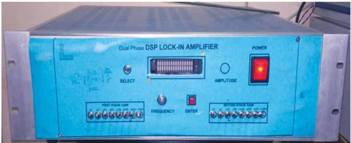
Fig. 3.1.11b: Analog front-end electronics and FPGA based digital back-end lock-in
