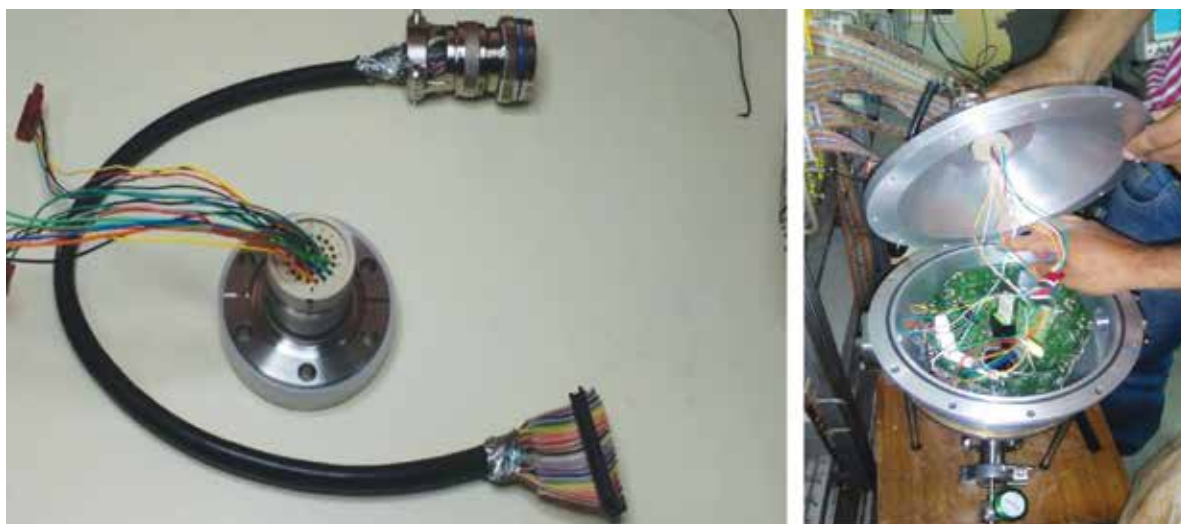
Fig 4.2.5: Left: 32 pin connector (air side plug on one side and vacuum side plug on another side) Right: In-situ view of chamber.
