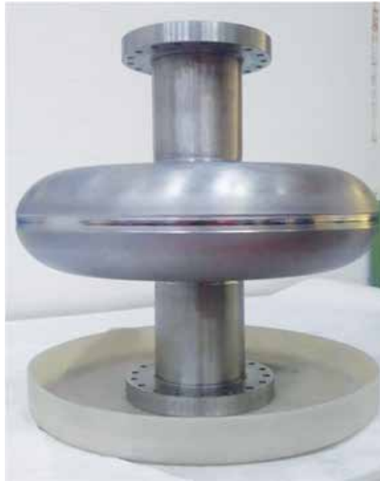
Figure 1.2.5: The second single cell 650 MHz, \beta=0.6 niobium LBC developed jointly by VECC and IUAC by adopting a procedure that is suitable for realizing multi-cell cavities.
