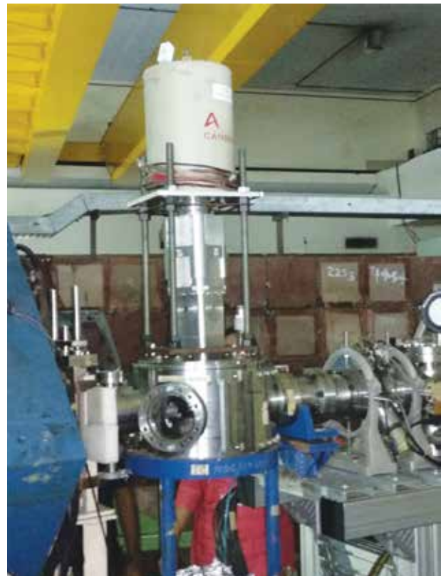
Fig.4.2.1 Clover detector mounted at the target site in HIRA beam line to study deep-sub-barrier reaction. The detector was at a distance of about 5 cm from the target.
