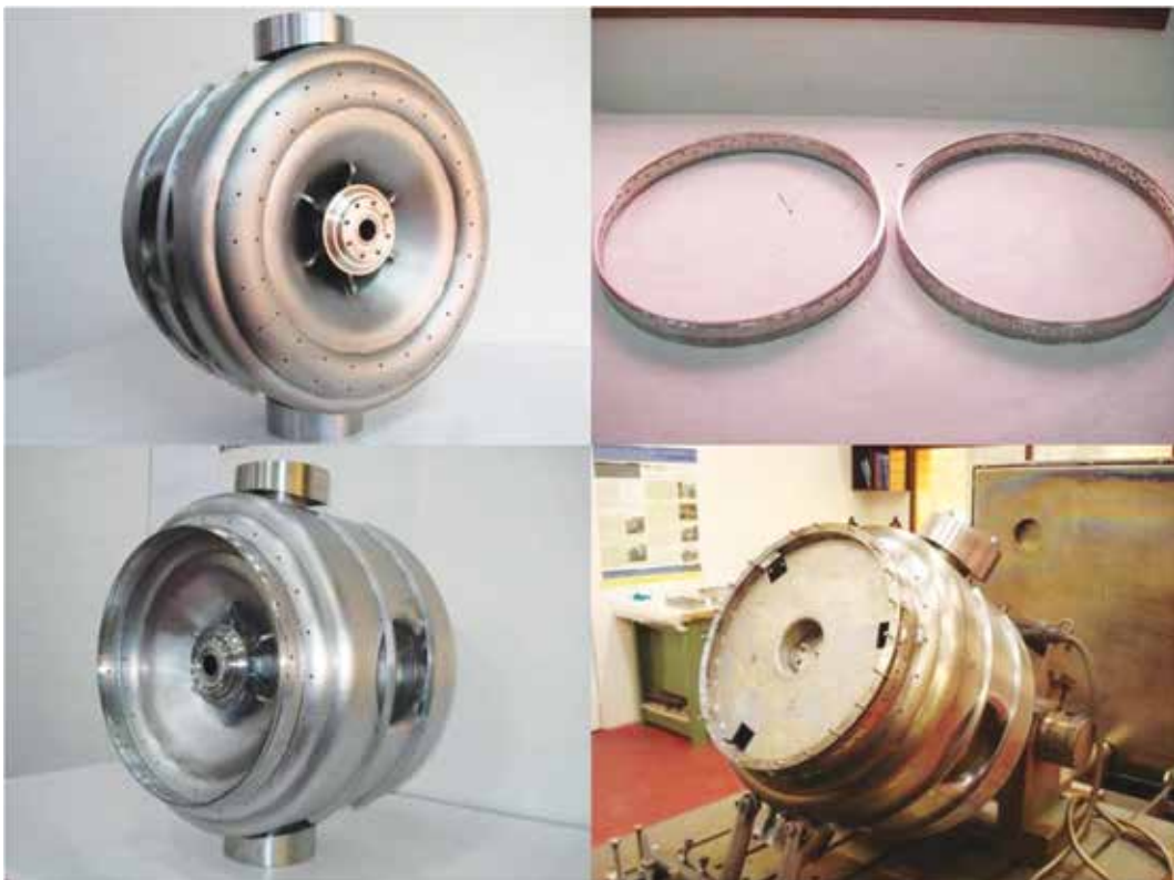
Figure 1.2.4: Clockwise from top-left: (i) SSR1 niobium single spoke resonator before attaching the Nb-SS brazed transition ring, (ii) Nb-SS brazed transition rings for the two SSR1 resonators, (iii) EBW set up for attaching the transition ring to the resonator, and (iv) SSR1 resonator after attaching the Nb-SS brazed transition ring just before sending to BARC, Mumbai, for the installation of the outer SS helium vessel.
