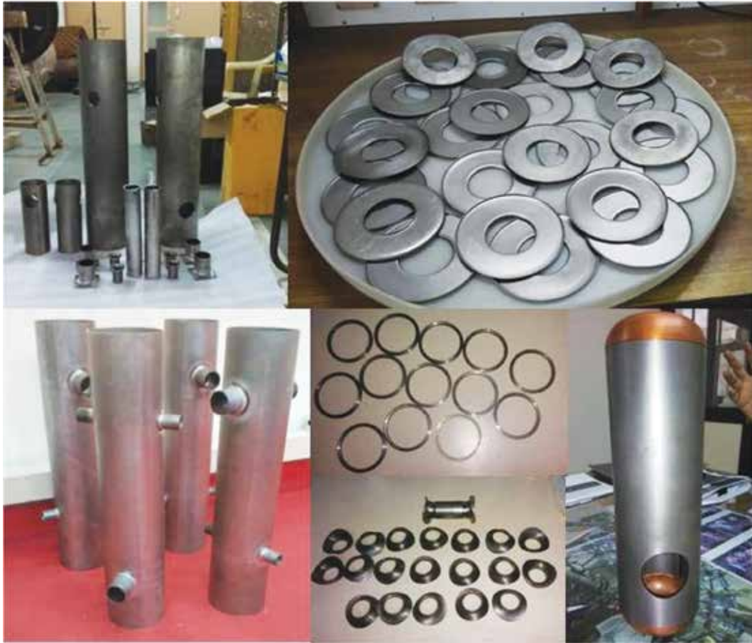
Figure 1.2.3: Clockwise from top-left: (i) niobium housings, drift tube cylinders, loading arms, coupling ports, beam ports etc., (ii) niobium leaves for the slow tuner bellows, (iii) drift tube cylinder with copper end caps (for checking the dimensions), (iv) top: slow tuner weld rings, (bottom): drift tube beam ports, (v) niobium outer housing cylinders.
