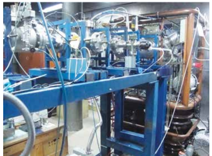
Fig. 10. View of the older version of the microwave ion source installed in the low energy facility.
