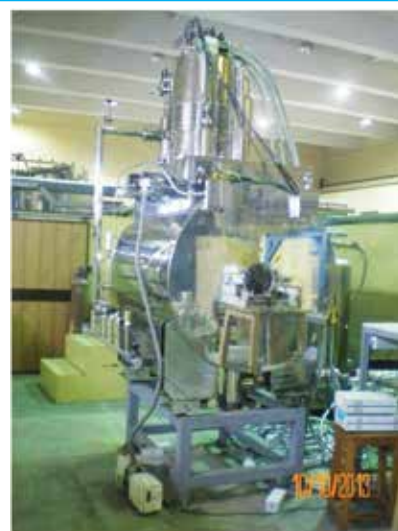
Fig. 2. Superconducting quadrupole magnet.
