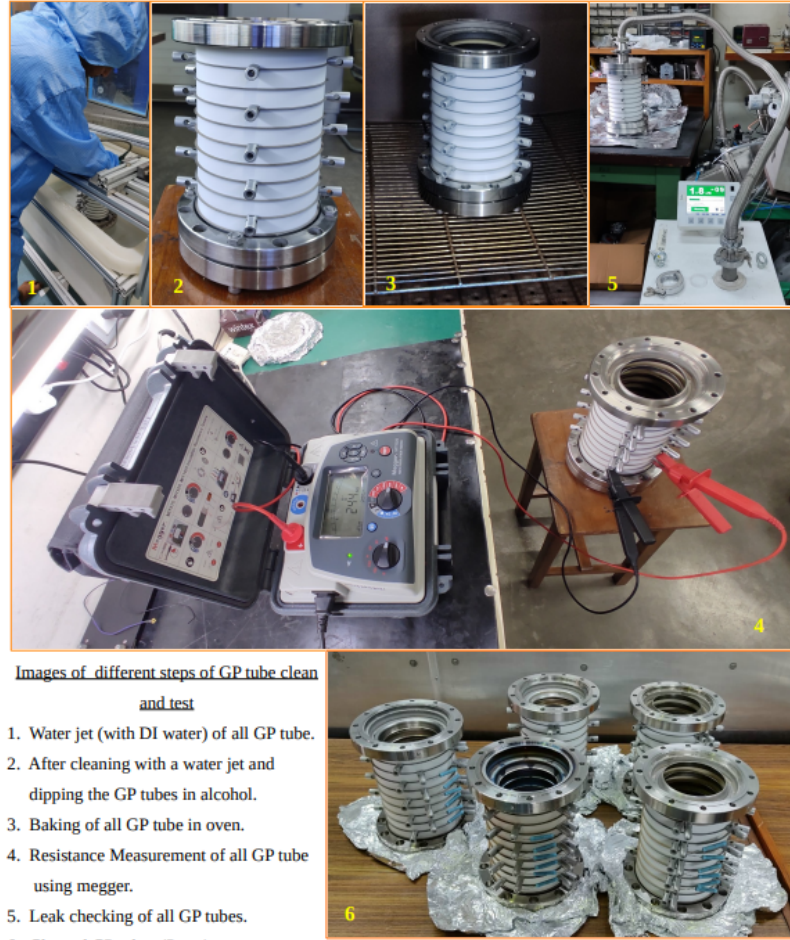
Figure 1.7: Steps followed for cleaning the GP tubes.
