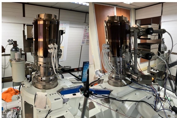
Figure 1.13: Baking of the column.
