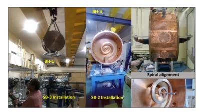
Figure 2.12: Photographs of installation of Spiral Buncher 2 and 3 in BH-3 and 1, respectively.
