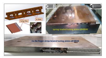
Figure 2.10: Photographs of burnt RF contacts of the RFQ frequency tuning plates.
