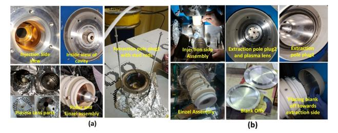
Figure 2.2: (a) View of the ion source parts before cleaning, (b) View of reinstalled parts of the ion source after cleaning.
